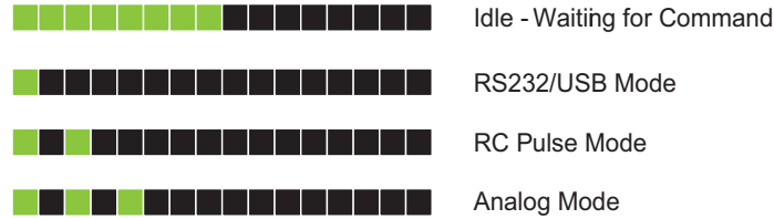
FIGURE 9. Normal Operation Flashing Patterns
