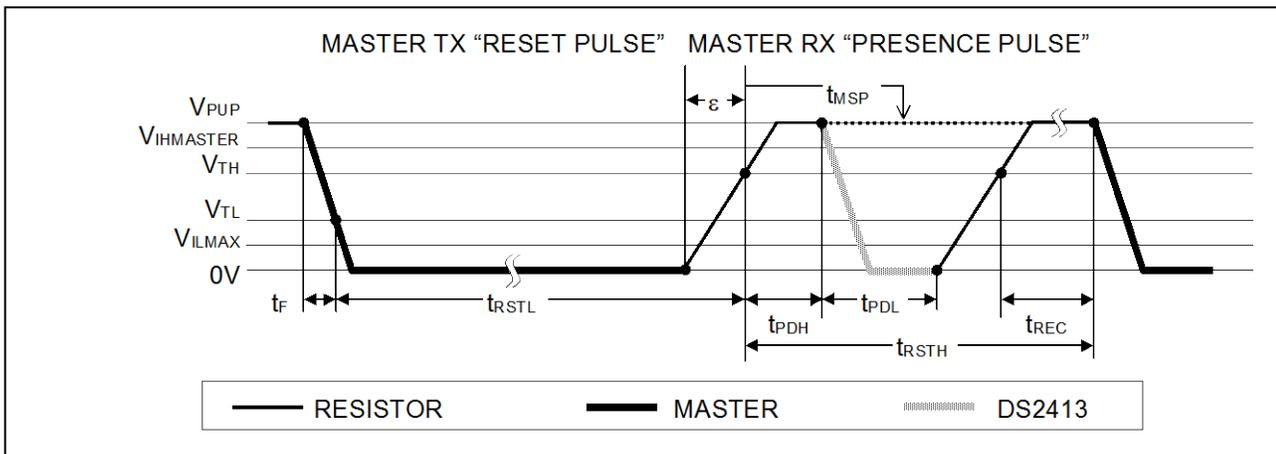
After the bus master has released the line it goes into receive mode. Now the 1-Wire bus is pulled to  $V_{PUP}$  through the pullup resistor, or in case of a DS2482-x00 or DS2480B driver, by active circuitry. When the threshold  $V_{TH}$  is crossed, the DS2413 waits for  $t_{PDH}$  and then transmits a Presence Pulse by pulling the line low for  $t_{PDL}$ . To detect a presence pulse, the master must test the logical state of the 1-Wire line at  $t_{MSP}$ .
